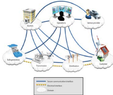
1. The basic conceptual model for the Smart Grid is useful in communicating the high-level concept. The detailed view in Figure 2 is messy, but vastly more informative.
